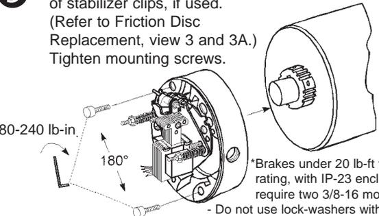
**6** AC coils are 50/60 Hz, single phase rated. Power supply to coil must not have current or frequency limiting output that is less than the coil requirement.
