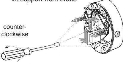
**3** Install new friction disc(s) and stationary disc(s) as shown.
