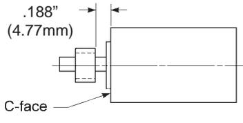
**3** Tighten set screws to motor shaft.
