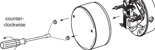
**5** Slide endplate over hub noting position of stabilizer clips, if used. (Refer to Friction Disc Replacement, view 3 and 3A.) Tighten mounting screws.
