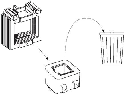
**7** A) Insert new coil. (Lead wires in same position as old coil.)
