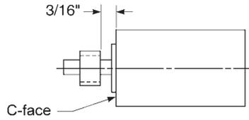
**3** Tighten set screws to motor shaft.
