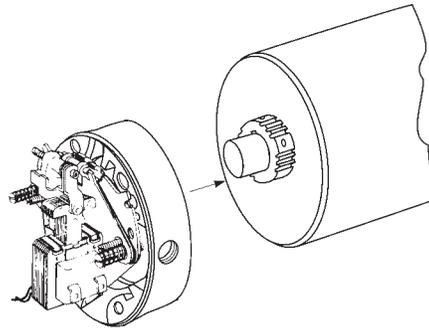
**6** Mount brake endplate to motor C-face.
