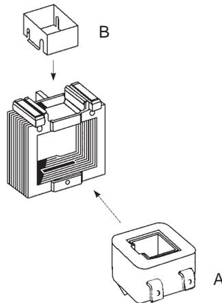
**8** A) Reinsert plunger into coil; drop pivot pin into cradle of support plate.
