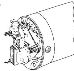
**3** Insert screwdriver between support plate and lever arm and pry forward.
