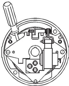
**4** Lift plunger/solenoid lever assembly out of coil.
