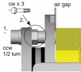
Air gap is factory set per Table D. Set air gap is measured at the adjusting bolts, between the armature and magbody.
