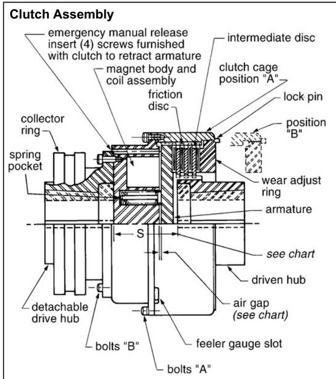
**CAUTION 1!** Thread manual release bolts into the armature and retract the armature against the magnet pole face before any disassembly of clutch.
