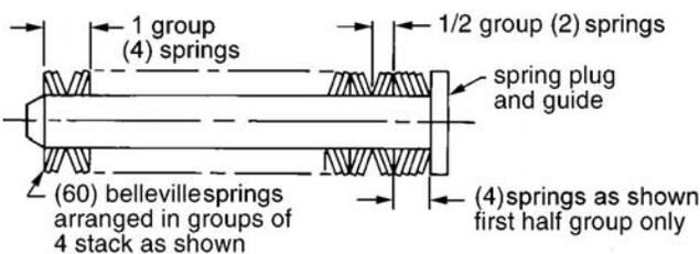
**Note:** Should removal of springs become necessary, they must be reassembled as shown to insure normal operation of clutch or brake.
