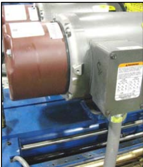
Picture: brake wired through to the motor with the brake motor connection diagram clearly identified on the junction box.
