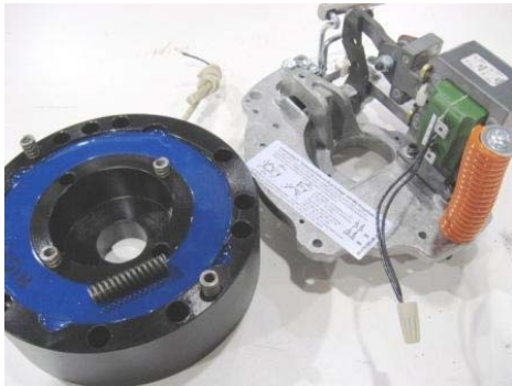
Picture 1: AAB magnet body with potted coil and a SAB support plate (1-087 series SAB shown).
