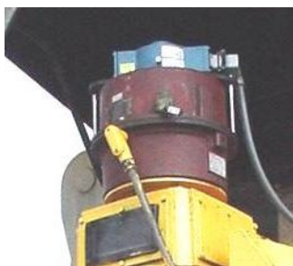
Picture one: An encoder is rigidly mounted to the brake housing. To inspect the brake, the encoder must be unbolted and removed. The through shaft is a potential leak path.
