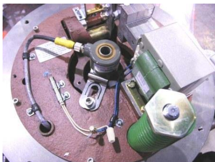
Picture five: The encoder cable is routed separately from the coil & heater.
