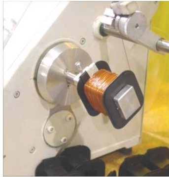
Picture 1: winding coil on a bobbin
